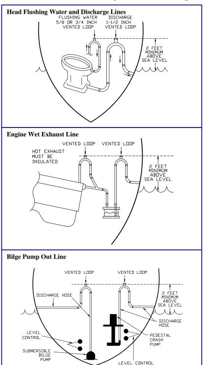
Type 890-913 Vented Loops include a sensitive marine vacuum breaker with a stainless steel spring to hold the poppet closed. A vacuum will pull the poppet open, permitting air to go into the system.
